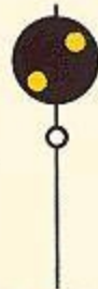
RULE 286 PROCEED AT MED- IUM SPEED PRE- PARING TO STOP AT NEXT SIGNAL
