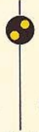
RULE 288 PROCEED PREPARING TO STOP AT NEXT SIGNAL. SLOW SPEED TO STOP SHORT WITHIN INTERLOCKING LIMITS.
