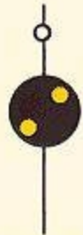
RULE 285 PROCEED PREPARING TO STOP AT NEXT SIGNAL. TRAIN EXCEEDING MEDIUM SPEED WHEN INDICA- TION IS SEEN MUST AT ONCE REDUCE TO THAT SPEED.
